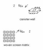
A conductive surface within the woven screen matrix models the radial heat flow in the screen wires and its "fin conduction length" input D recast to one-quarter the canister diameter (D = 0.25 \* Din). (See sample problems in the Stirling Manual for more discussion about why.)
