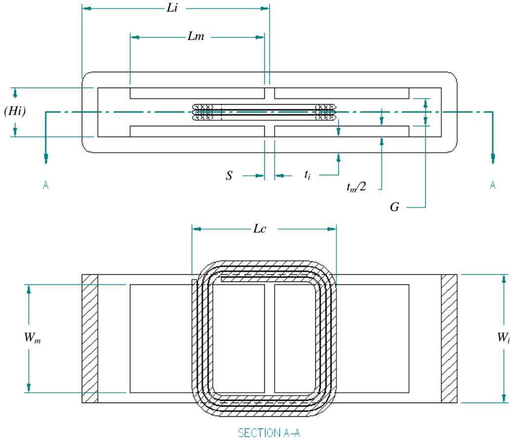
In the model  $L_m$ ,  $S$ ,  $G$  and  $W_m$  set the dimensions of the *two-pole magnetic gap* via input recasts. The length of the moving container inside the gap is recast to coil length  $L_c$ . The offset of the container at the center position is recast to
