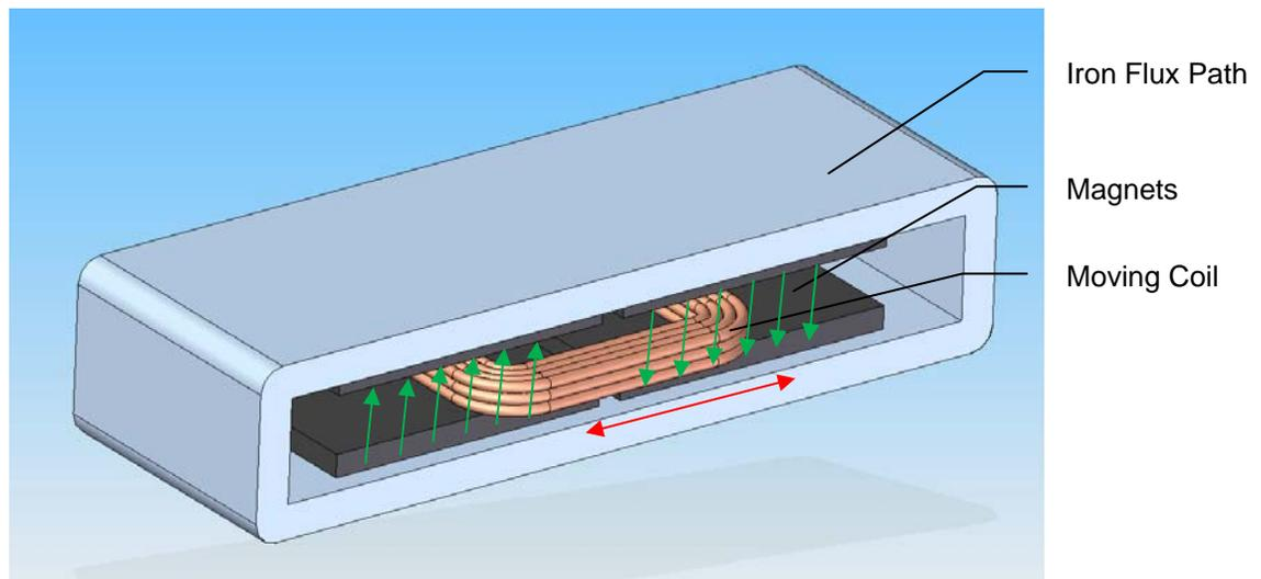
The structure that actually moves and aligns the coil is not shown. In hard-drive practice the coil moves along an arc rather than a straight line and the magnets and iron structure are curved accordingly.
