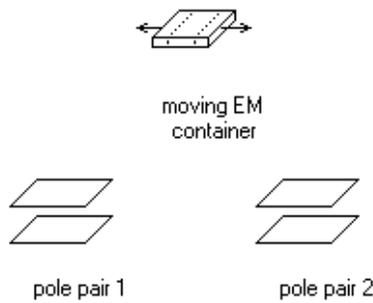
The idea is that whatever is inside the *moving EM container* passes between pole pairs 1 and 2 and sees opposite magnetic flux.
