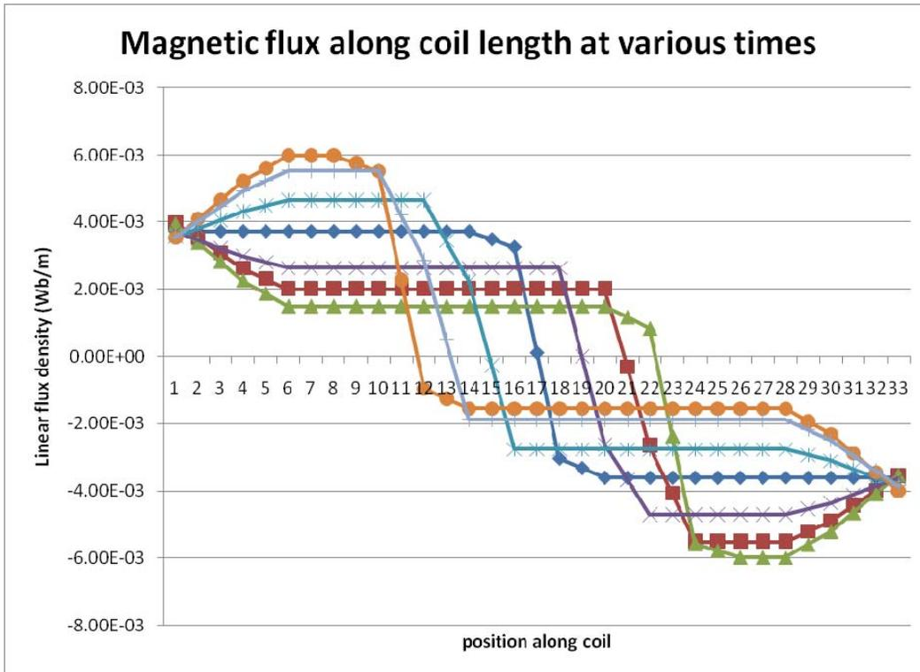
The cross-legs (across the gap) of the coil winding occupy the left and right ends of the plot where the curves are sloped. The magnetic field produced by the current in the coil changes the baseline magnetic flux produced by the permanent magnets alone. That baseline magnetic flux can be seen in the middle curve which corresponds to the time of zero electrical current. Baseline magnetic flux goes from a positive to a negative value across the gap separating the oppositely polarized magnets.
