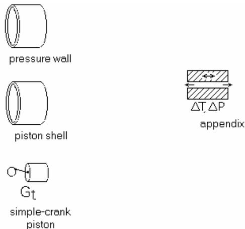
The *appendix* models the annular gas gap between the piston dome and cylinder wall, including the combined conduction of the two walls and the shuttle heat transfer mechanism produced by the thermal interaction between them as they move relative to
