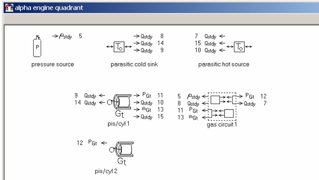
The *pressure source* establishes the mean cycle pressure.
