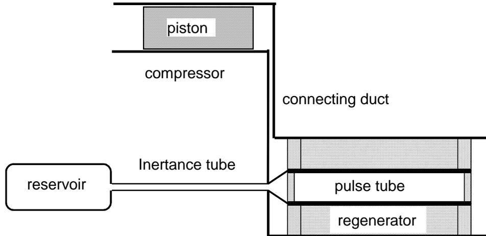
At the top-level the Sage model consists of a compressor submodel and a cold-head submodel with a connecting duct between the two:
