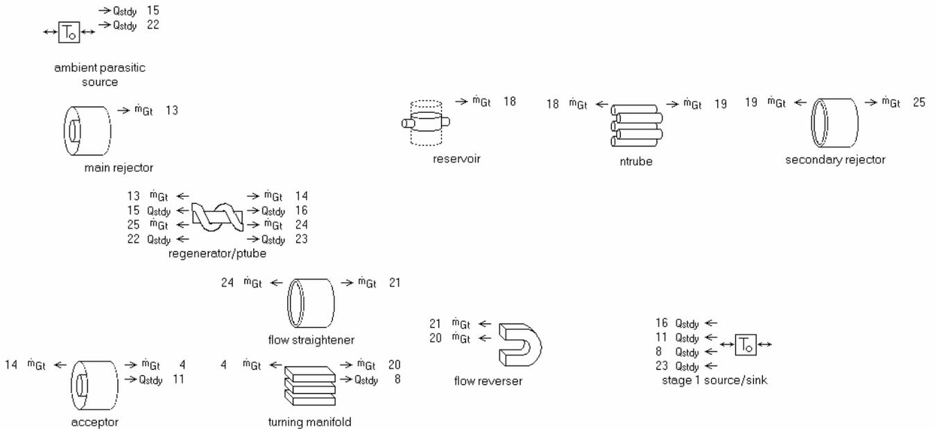
The regenerator and pulse-tube are housed within the multi-length container *regenerator/ptube*, which looks like this inside:
