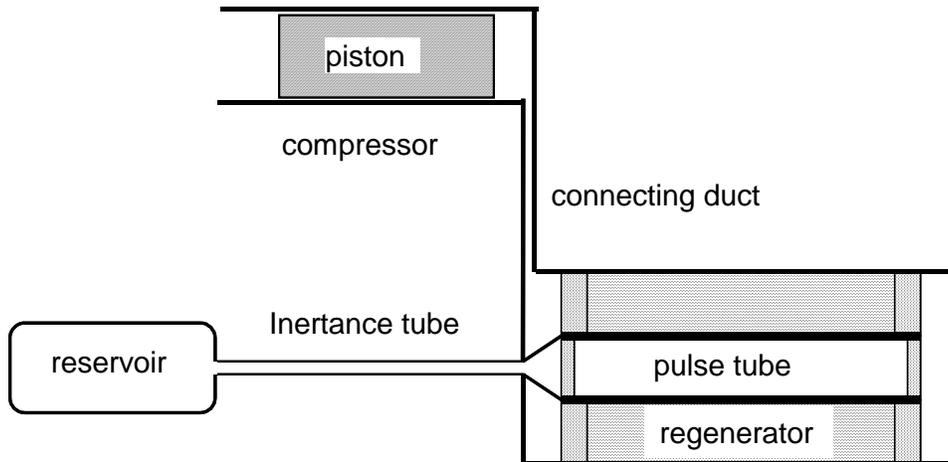
This model derives from the CoAxPTR model and inherits most of its structure except for the packaging of the regenerator and pulse tube within the cold head. This document discusses only the new features compared to the CoAxPTR model and is a supplement to the original documentation found in file CoAxPTR.pdf.
