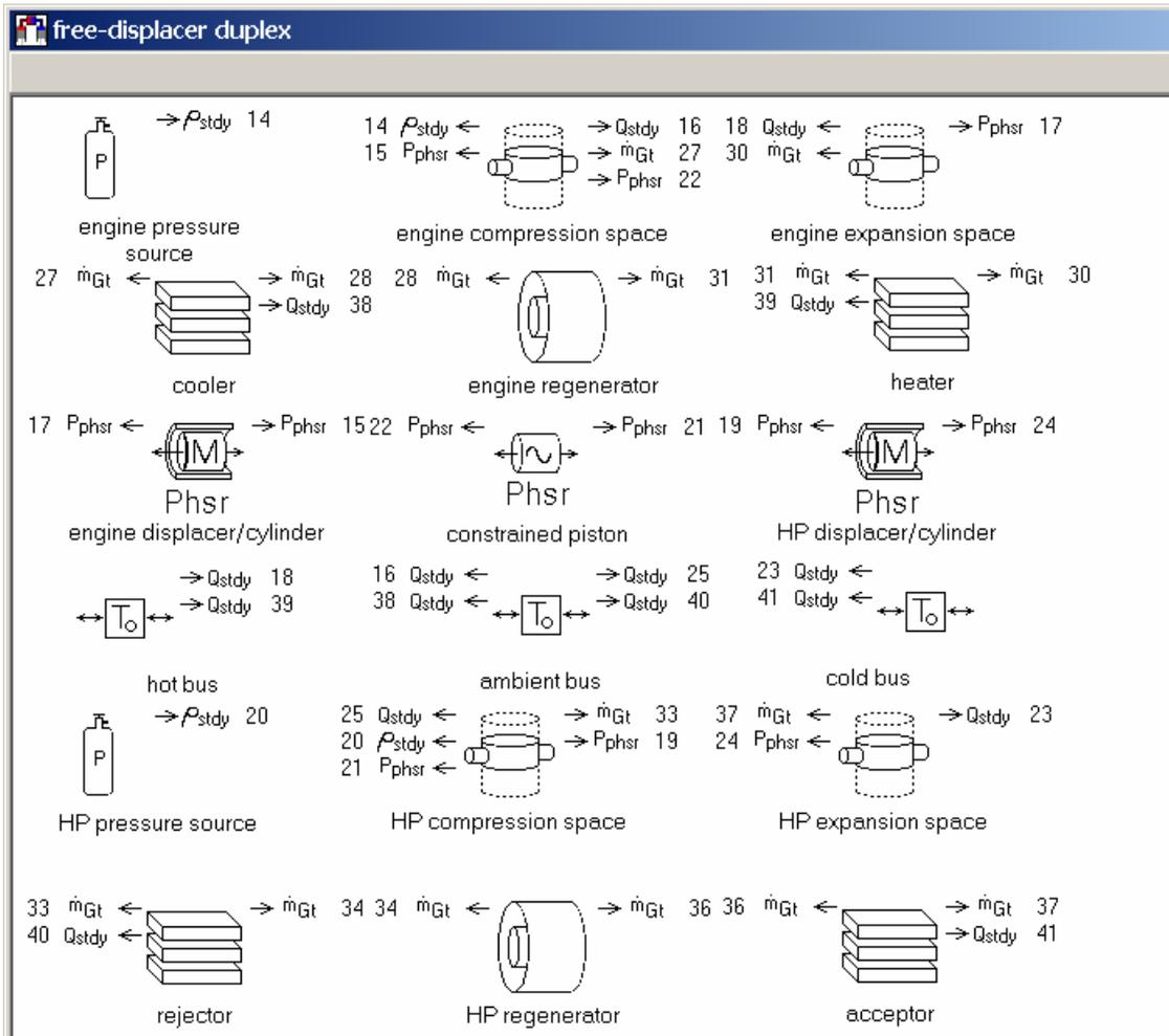
The engine components are at the top and the heat pump components at the bottom, separated by the *constrained piston* and two *displacer/cylinder* components in the middle. The orientations of the heat pump, piston and displacer/cylinder components are faithful to the orientation of the schematic but the engine components are flipped around so that the hot end is toward the right (positive direction) instead of the left.
