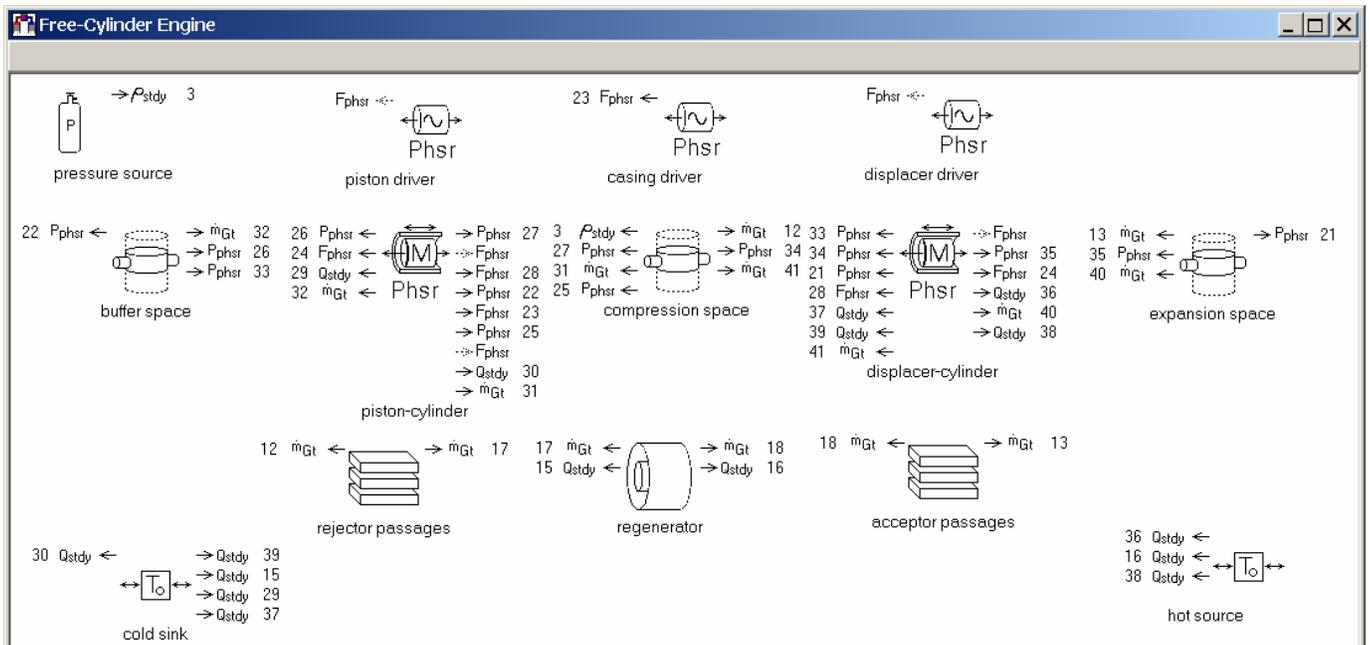
In the model the casing is not actually free. The *casing driver* component forces it to move at a specified amplitude and phase ( $Xamp$  and  $Xphase$  inputs) and the load is represented only in terms of the forcing function  $FF$  required to absorb the total mechanical power delivered to the casing, eventually the result of the PV power delivered by the working gas to the compression and expansion space boundaries.  $FF$  is an output variable of the *cylinder driver* component.
