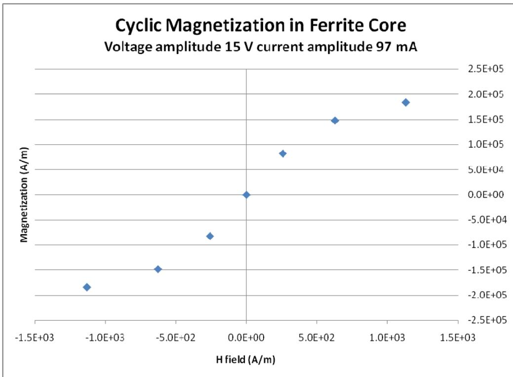
The magnetization traces the familiar curve except there is no discernable hysteresis because the coercive force (H intercept of magnetization) is only about 0.5 A/m for ferrite. Sage soft ferromagnetic material output Whyst reports only 0.27 mW loss for this case.
