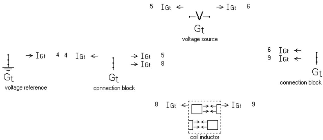
A voltage source (top row) drives electrical current through a coil inductor submodel where the resistance and inductance come from coil and soft ferromagnetic material components shown here
