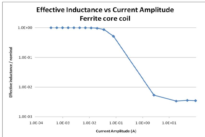
The model inductance compares well with the expected theoretical value until current amplitude reaches about 10 mA after which it declines rapidly to the air-core value, which is  $1/350 = 2.86E-3$  in relative terms.
