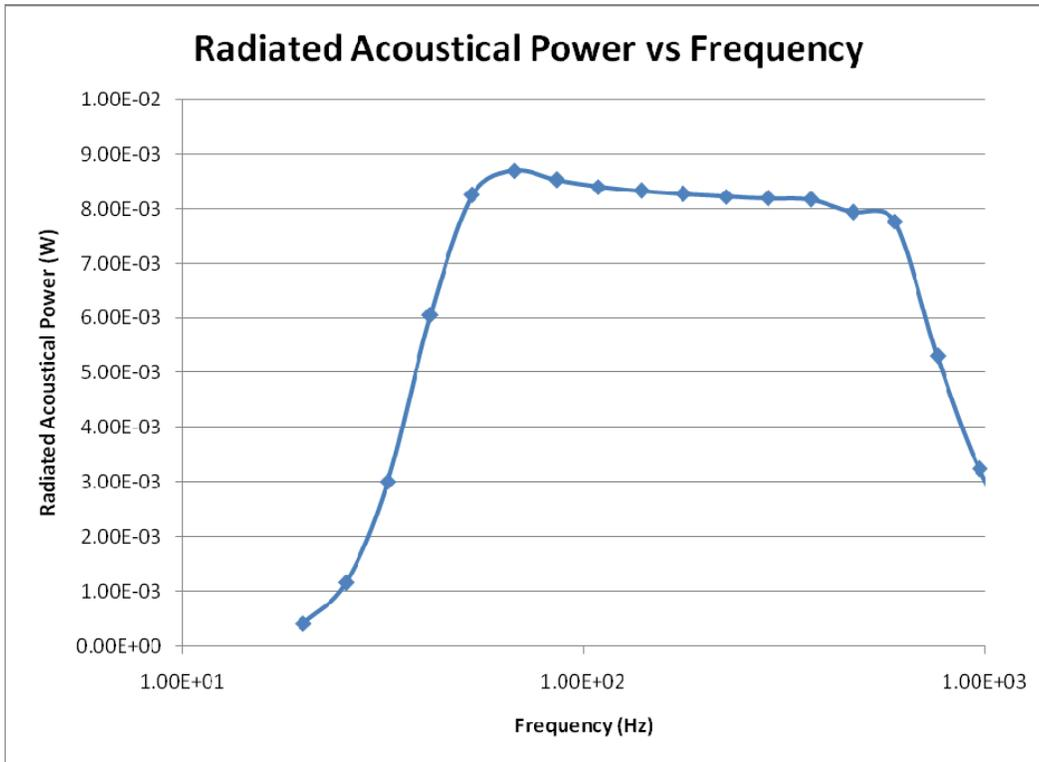
A sharp peak at the 41 Hz mechanical resonant frequency is eliminated by choice of the damping coefficient (40 N s/m) of the *suspension damper* component. That is about half the critical damping ratio of 77 Ns/m, given by the standard formula
