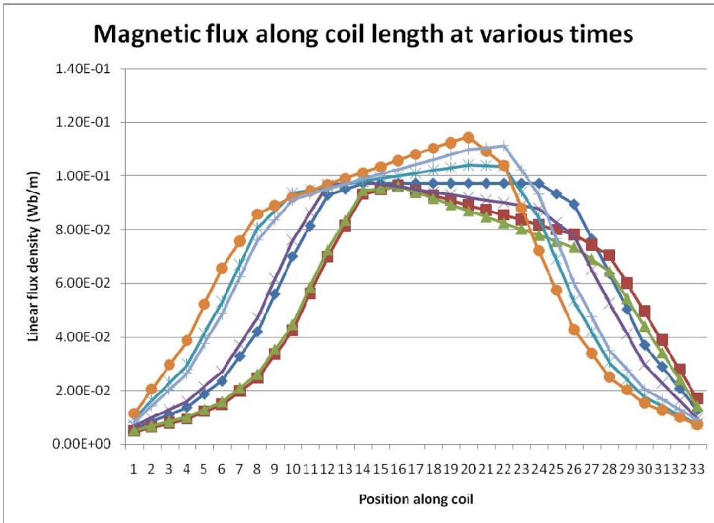
The magnetic flux is highest for the part of the coil between the pole faces and drops off on either side according to the fringing flux formulation in Sage. The reason the location of the highest magnetic flux moves back and forth is because the plot is in the coil reference frame from which the outer magnetic structure appears to be moving back and forth.
