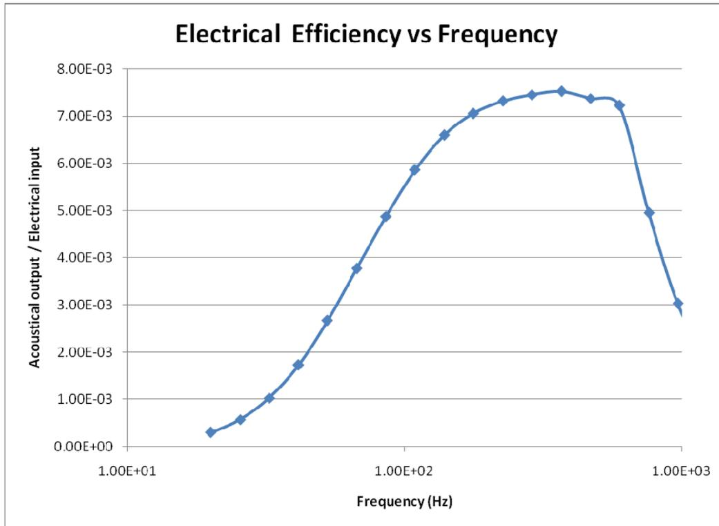
Electrical efficiency is defined as time-average electrical input power / acoustical power output, which is available in the model via user-defined variables *Wacous* in the *speaker cone*, *Welec* in the *current source* and *Effic* in the root model. The peak efficiency is about 0.75% at about 400 Hz.
