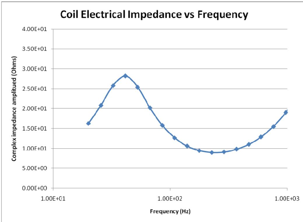
According to Wikipedia<sup>2</sup> the nominal impedance of a loudspeaker is 1.15 time higher than the minimum impedance along the frequency curve. So the loudspeaker in the model has a nominal impedance of about 10.4 ohms (minimum impedance 9.0 ohms).
