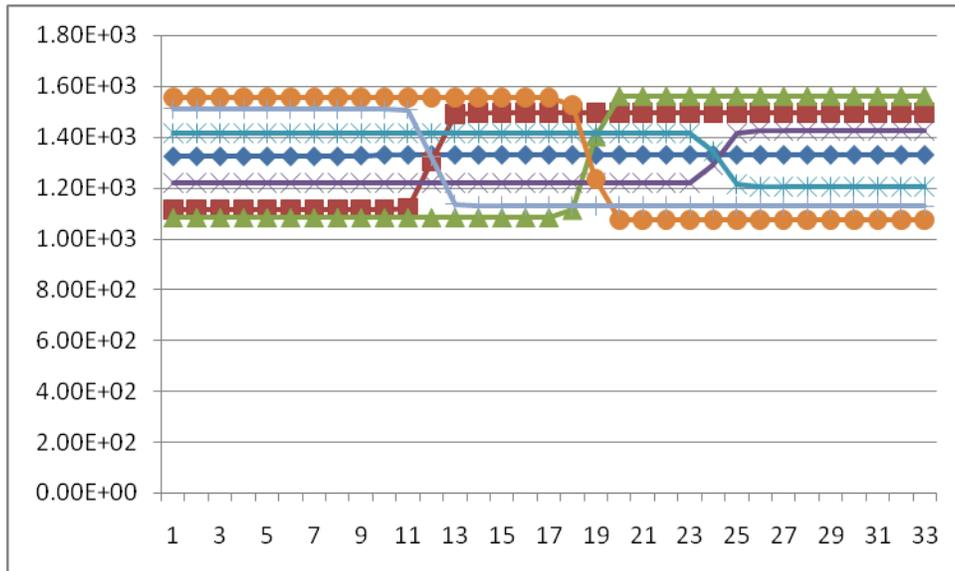
Where each curve represents a different time and the horizontal axis corresponds to position along the magnet. The point where external potential shifts between pole 1 and pole 2 values shifts back and forth. That is because the data is in the magnet reference frame in which the outer poles are moving back and forth.
