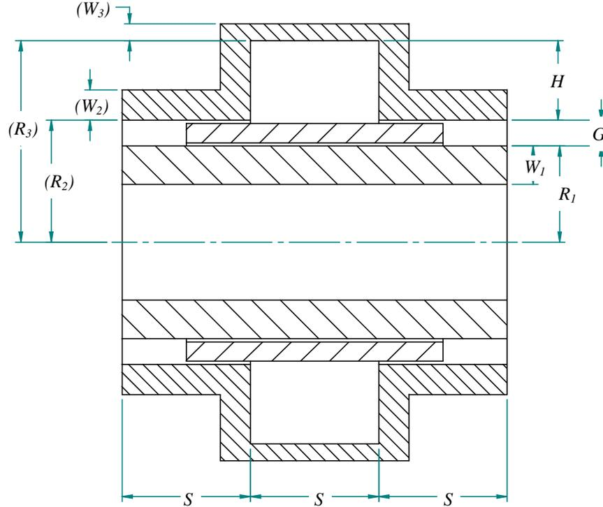
For simplicity the pole pieces and coil space all have the same length  $S$ . In this model  $S$  is twice the design point magnet amplitude. The magnet is drawn at its center position. So at its extreme negative (left) position the magnet fully fills the gap of pole pair 1 and likewise for the gap of pole pair 2 at the extreme positive position.
