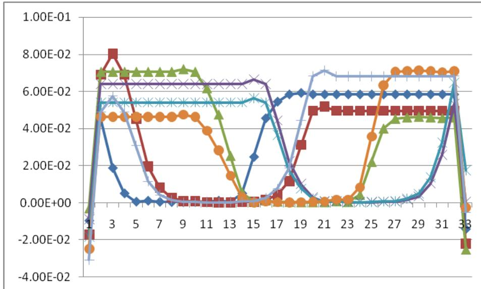
The magnetic flux drops off to near zero in the space separating the poles but not abruptly because Sage approximately models the fringing field outside the pole nominal boundaries.
