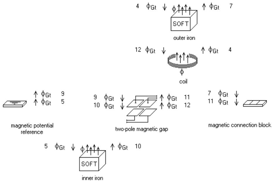
Admittedly the Sage motor submodel looks nothing like the actual motor. The inner and outer iron pieces are represented by two linear paths connected in series with each other and the coil across the two pole pairs of the *two-pole magnetic gap*. Tracing connection arrows shows this is so.
