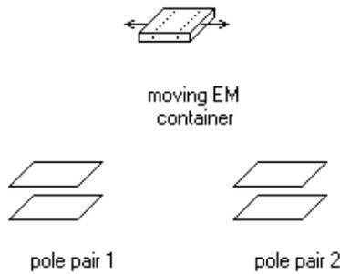
The idea is that the magnet inside the moving EM container passes between pole pairs 1 and 2 and drives flux through the external magnetic path accordingly.
