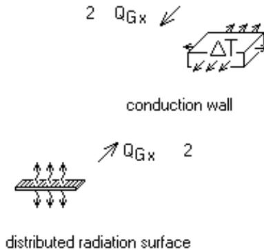
The heat flow connection  $Q_{Gx}$  anchors the *distributed radiation surface* temperature to the *conduction wall* temperature distribution. The *conduction wall* temperature is solved according to the energy balance between axial thermal conduction down the wall and distributed radiation heat transfer.
