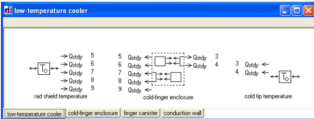
The *rad shield temperature* anchors all the radiation shield surfaces and one end of a cylindrical canister wall (thermal solid) representing the cold finger pressure wall. The
