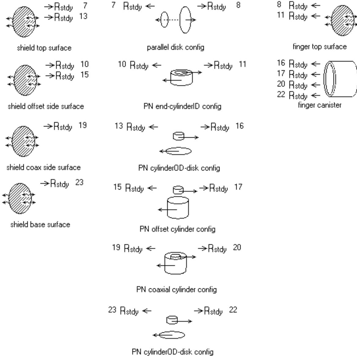
The radiation shield surfaces are in the left column and the cold finger surfaces in the right column. Between the two columns are all the view configurations by which the radiation shield surfaces see the cold finger surfaces. The view configurations between individual surfaces of the radiation shield are not included in the model because they are at the same temperature and there is no net radiation exchange between them.
