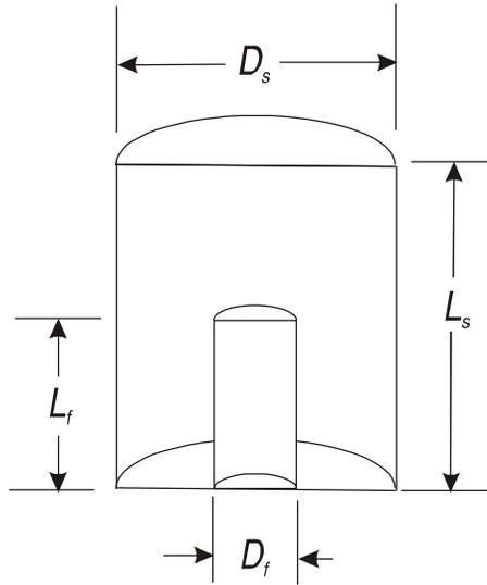
The interesting thing about this model is that the cold finger cylinder has a temperature distribution ranging between the cold-tip temperature and the radiation shield temperature. All the other surfaces have uniform temperatures. Of interest is the net radiation exchange between the radiation shield and cold finger.
