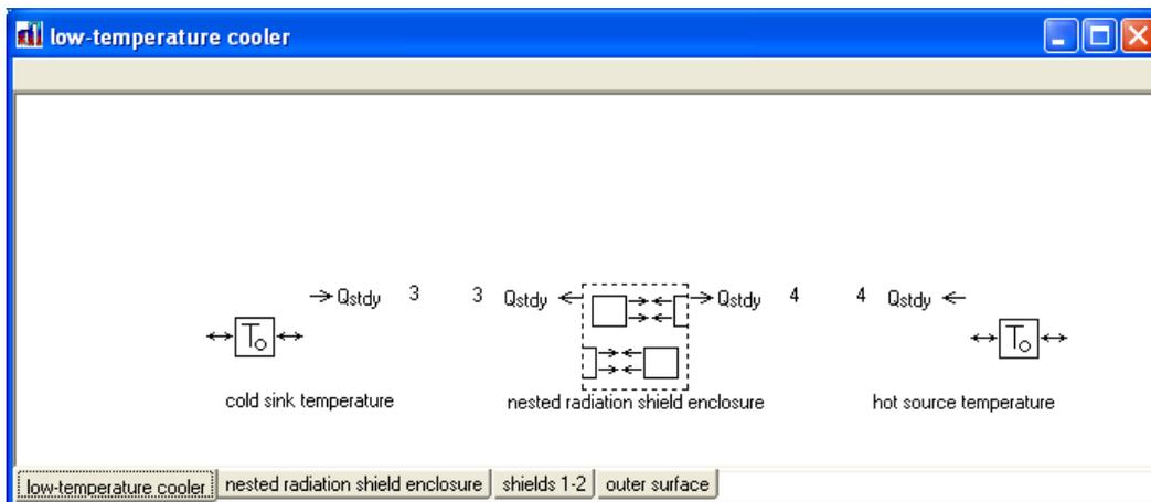
The *cold sink temperature* and *hot source temperature* anchor the two ends of the radiation shields located within the *nested radiation shield enclosure* submodel.
