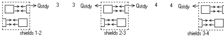
It is possible to increase the number of shields by disconnecting one of them and copy/pasting any number of times. The actual radiation exchange components within any one of the *shields* submodels are shown here:
