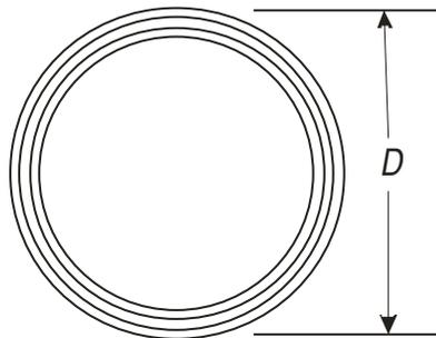
The inner and outer surfaces are anchored to external fixed temperatures. Of interest is the net radiation exchange between them. The inner two shields float in temperature. With fixed temperatures the inner shield might actually represent the surface of some payload that is to be insulated and the outer surface a container wall in good thermal contact with the ambient temperature. In which case there are only two actual radiation shields.
