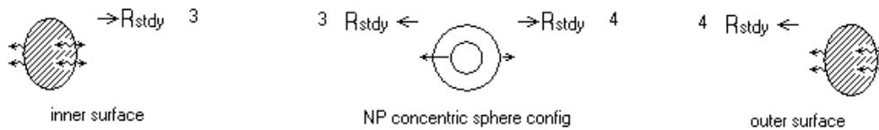
The *inner surface* and *outer surface* have ordinary (conductive) heat flow connections moved up to the submodel level for connection to a radiation surface of another *shield* submodel or to one of the root-level temperature sources. Connecting a shield surface to a temperature source fixes its temperature. Connecting two shield surfaces together forces their temperatures to be equal but allows both to float as part of the solution.
