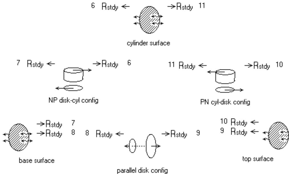
The *base surface* and *top surface* have ordinary (conductive) heat flow connections moved up to the submodel level for connection to a radiation surface of another *shield* submodel or to one of the root-level temperature sources. Connecting a shield surface to a temperature source fixes its temperature. Connecting two shield surfaces together forces their temperatures to be equal but allows both to float as part of the solution.
