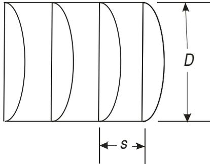
Displacers of stirling machines often contain radiation shields when not serving as a regenerator housing. This model simulates only the radiation heat transfer within such a displacer, not the thermal conduction within solid walls.
