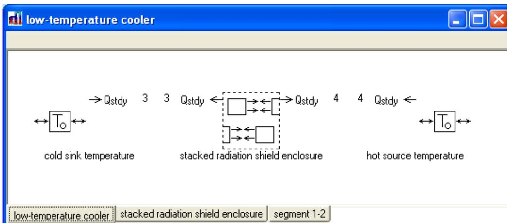
The *cold sink temperature* and *hot source temperature* anchor the two ends of the radiation shields located within the *stacked radiation shield enclosure* submodel.
