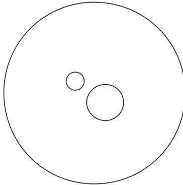
All three spherical surfaces are anchored to external fixed temperatures. Of interest is the net radiation exchange to each surface.
