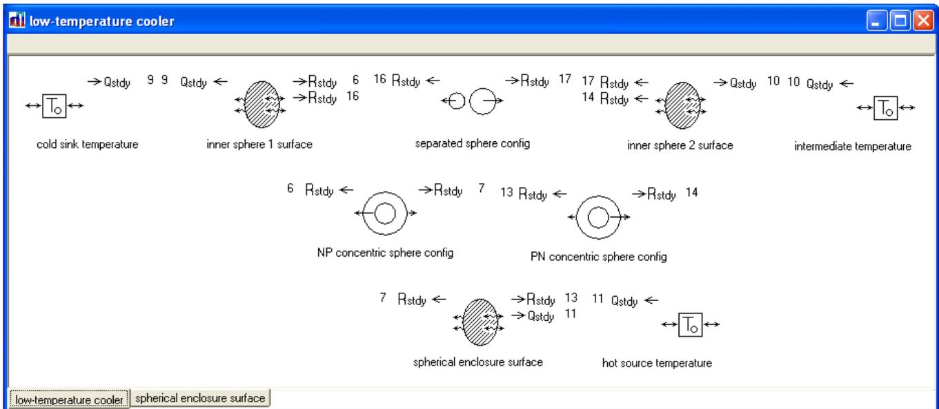
It is only an approximate model. The concentric-sphere view configuration connecting each inner sphere to the surrounding enclosure does not consider the partial blocking of the view by the other inner sphere. The *hot source temperature* anchors the *spherical enclosure surface* at 300 K. The *cold sink temperature* and *intermediate temperature*
