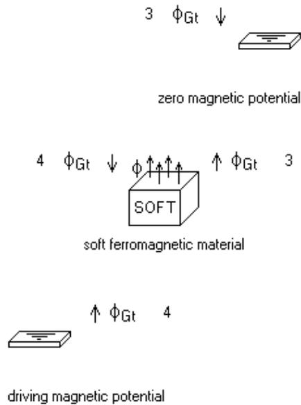
A driving magnetic potential produces a magnetic flux through a soft ferromagnetic material anchored by a zero magnetic potential at the positive (upper) end.
