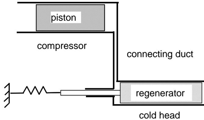
The Sage model consists of the compressor, connecting duct and cold-head components all within the top level model:
