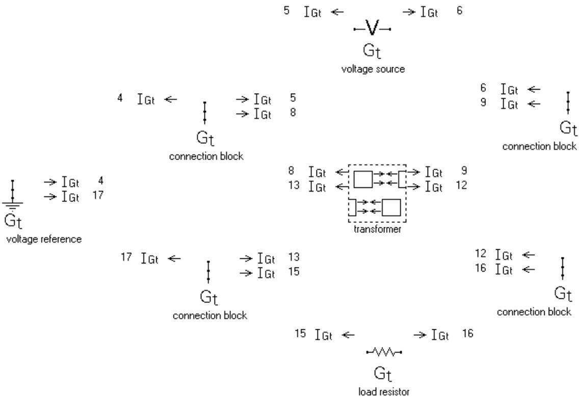
A voltage source (top row) drives electrical current through the primary winding within the transformer submodel. The secondary winding drives current through the load resistor. Within the transformer submodel are these components:
