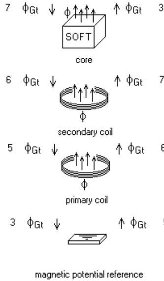
The two coils and core (ferromagnetic material) form a magnetic circuit anchored by a magnetic potential reference. Electrical current flowing through the primary coil produces a magnetic field that drives magnetic flux through the secondary coil. Actually, both coils produce magnetic fields that combine to produce magnetic flux through the core that links both coils.
