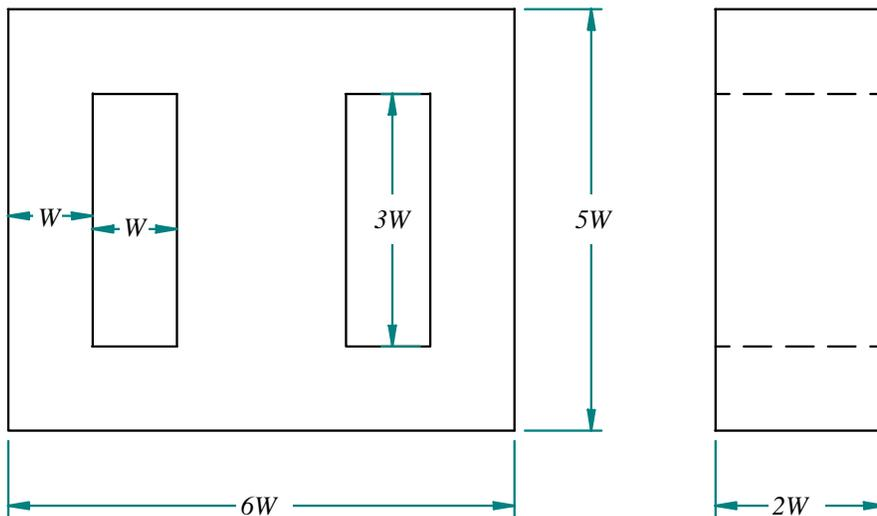
The coils are wound through the rectangular cutouts. Fluctuating current in the coils drive magnetic flux up (or down) the central leg where it splits to form two loops directed down (or up) the outer legs and returning to the central leg. In the Sage model these two flux loops are combined into a single one-dimensional path of cross-section area equal to the central leg cross section and length equal to the mean length of the path around one of the cutouts.
