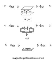
The coil and air gap form a magnetic circuit anchored by a magnetic potential reference. Electrical current flowing through the coil produces a magnetic field that drives magnetic flux through the air gap. The changing magnetic flux induces a counter EMF in the coil that opposes the current change.
