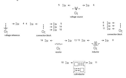
A voltage source (top row) drives electrical current through two circuit elements in parallel. One circuit element (third row) is a simple resistor and inductor in series where the resistance and inductance are set as inputs. The other circuit element is a coil inductor submodel (bottom row) where the resistance and inductance come from coil and air-gap components. The contents of the coil inductor submodel are these:
