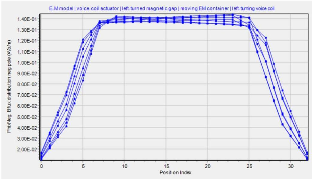
The magnetic flux is highest for the part of the coil between the pole faces and drops off on either side according to the fringing flux formulation in Sage. The reason the location of the highest magnetic flux moves back and forth is because the plot is in the coil reference frame from which the outer magnetic structure appears to be moving back and forth.
