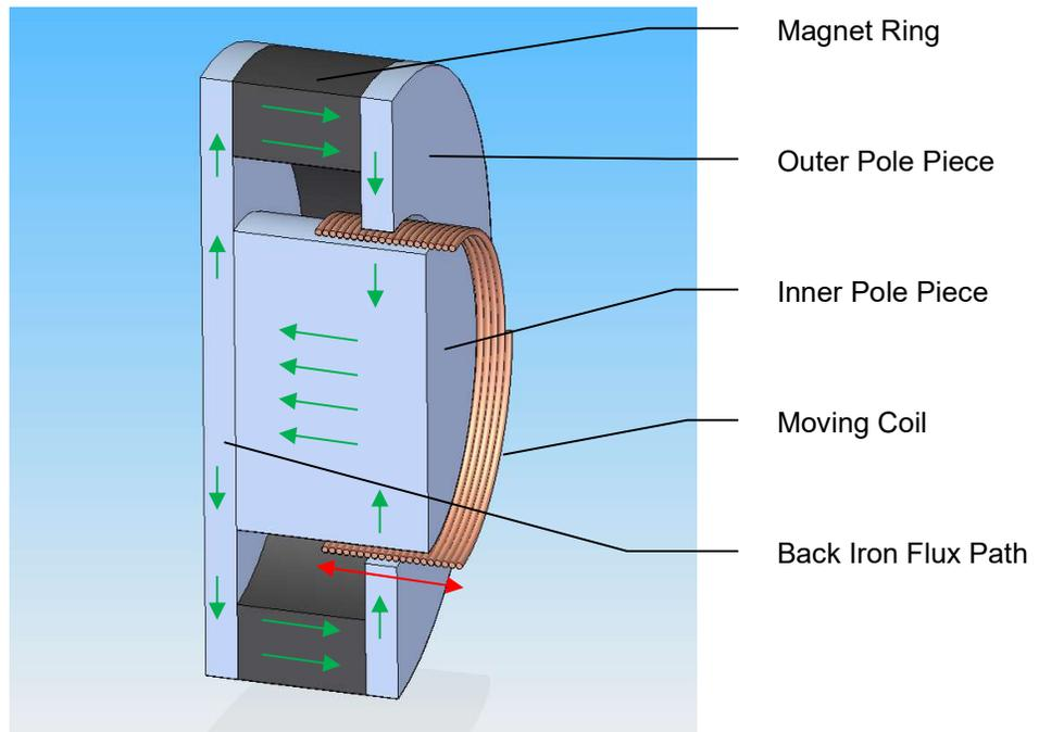
The voice coil is longer than the air gap so that it remains entirely within the gap during normal operation and produces a linear variation of actuator force with electrical current, independent of coil position. The speaker cone attached to the coil and outer structure that holds everything in alignment is not shown.
