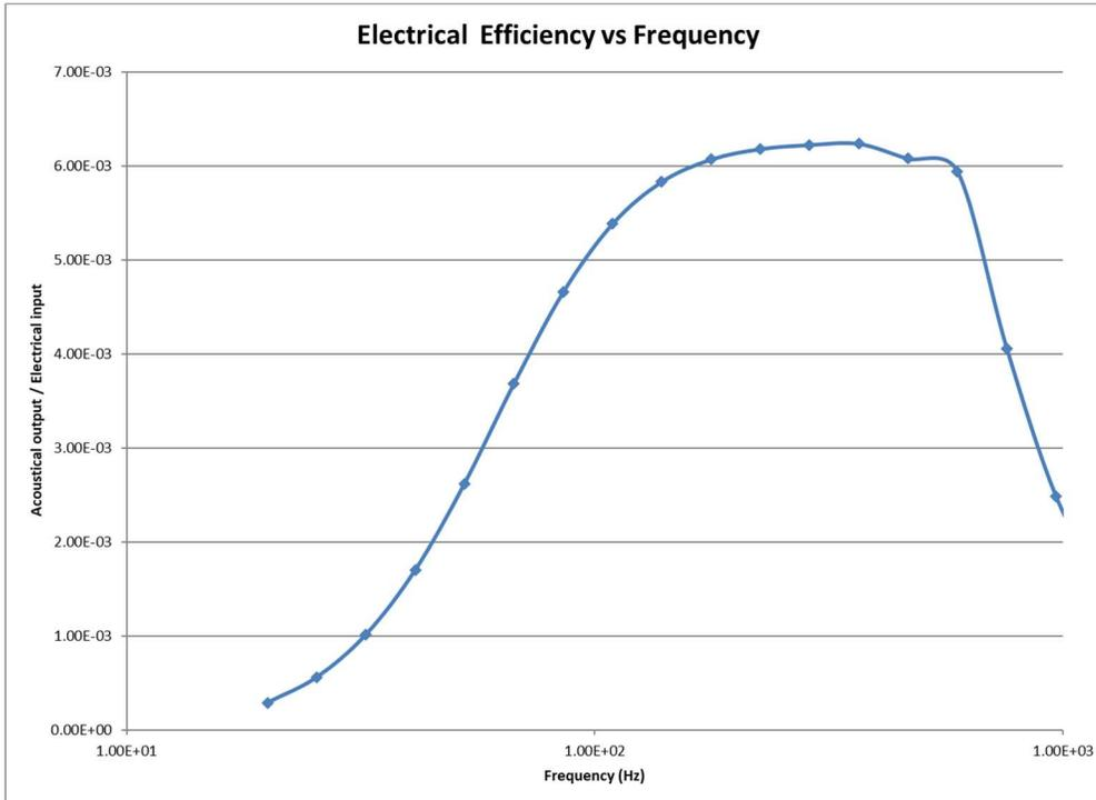
Electrical efficiency is defined as time-average electrical input power / acoustical power output, which is available in the model via user-defined variables  $W_{acous}$  in the *speaker cone*,  $W_{elec}$  in the *current source* and  $E_{ffic}$  in the root model. The peak efficiency is about 0.62% at about 400 Hz.
