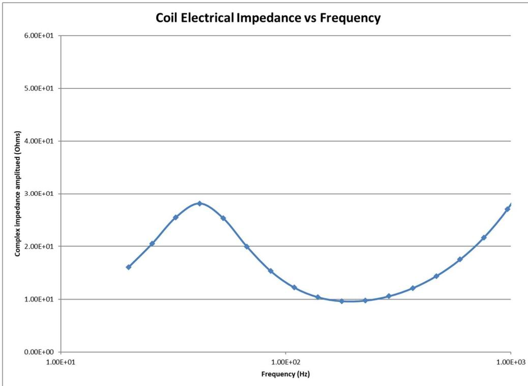
According to Wikipedia<sup>2</sup> the nominal impedance of a loudspeaker is 1.15 times higher than the minimum impedance along the frequency curve. So the loudspeaker in the model has a nominal impedance of about 11 ohms (minimum impedance 9.6 ohms).
