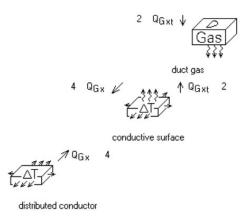
The duct gas and conductive surface components are the same as in the HeatExchangers-SimpleIsothermal.scfn sample model and will not be discussed further here.
