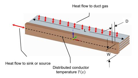
Sage solves the distributed-conductor temperature T(x) based the thermal conductivity and heat flow equations within the distributed conductor and the thermal boundary conditions provided by the temperature of the source or sink attached to the left endpoint and the temperature of the gas attached to the fin faces.
