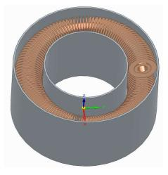
In Sage, the model uses the *multi-length container*, *tubular bundle, rectangular fins* and two instances of the *distributed conductor* components, except they are renamed *circumferential finned tube recuperator*, *tubes*, *circumferential fins*, *tube walls* and *fin path*:
