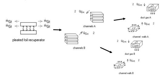
The  $Q_{Gx}$  connectors between the *channels A* and *B* components are bumped up one level from the *channel walls A* and *B* within.
