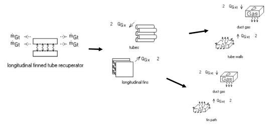
The  $Q_{Gx}$  connectors between the *tubes* and *longitudinal fins* components are bumped up one level from the *tube walls* and *fin path* within.
