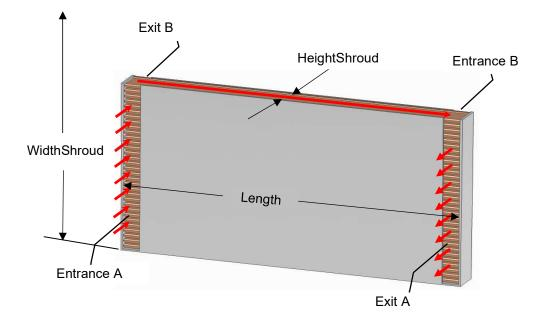
This model might form the basis for an air preheater in a combustion system where both fluid streams are near atmospheric pressure and there is no structural loading on the flat plates.
