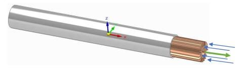
In Sage, the model uses the *parallel container*, *tubular bundle, rectangular fins* and two instances of the *distributed conductor* components, except they are renamed *longitudinal finned tube recuperator*, *tubes, longitudinal fins, tube walls* and *fin path*:
