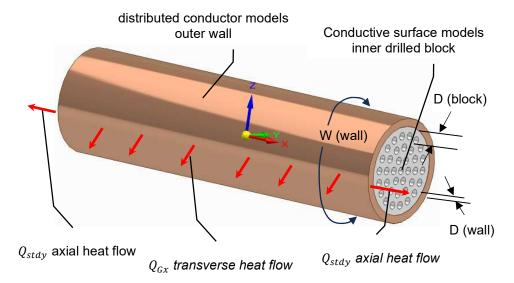
The  $Q_{stdy}$  connections can be used to transfer heat through the outer wall ends. The  $Q_{Gx}$  connection can be used to transfer heat through the outer wall cylindrical surface. One option is to attach the  $Q_{Gx}$  connector to a line heat source or line heater component with temperature or heat flux adjusted based on a separate analysis of external heat transfer.
