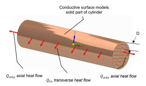
The  $Q_{stdy}$  connections can be used to transfer heat through the block ends. The  $Q_{Gx}$  connection can be used to transfer heat through the outer cylindrical surface. One option is to attach the  $Q_{Gx}$  connector to a line heat source or line heater component with temperature or heat flux adjusted based on a separate analysis of external heat transfer. See below for other options.
