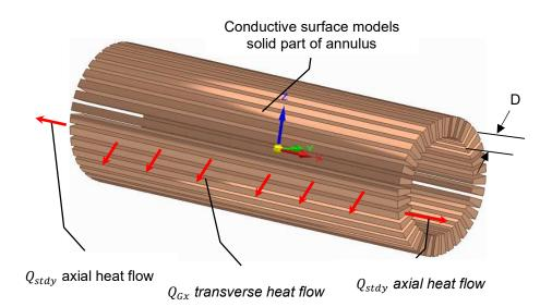
The  $Q_{stdy}$  connections can be used to transfer heat through the annulus ends. The  $Q_{Gx}$  connection can be used to transfer heat through the outer cylindrical surface (all fins simultaneously). One option is to attach the  $Q_{Gx}$  connector to a line heat source or line heater component with temperature or heat flux adjusted based on a separate analysis of external heat transfer.
