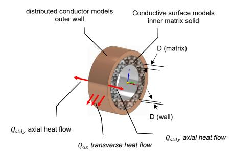
The  $Q_{stdy}$  connections can be used to transfer heat through the outer wall ends. The  $Q_{Gx}$  connection can be used to transfer heat through the outer wall cylindrical surface. One option is to attach the  $Q_{Gx}$  connector to a line heat source or line heater component with temperature or heat flux adjusted based on a separate analysis of external heat transfer.
