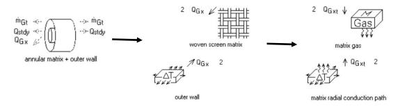
The matrix-radial-conduction path  $Q_{Gx}$  connector has been bumped up one level for connection to the outer wall.
