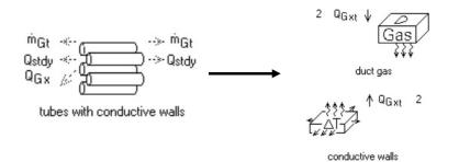
According to the actual geometry, the model renames the *tube bundle* component to *tubes with conductive walls* and the *conductive surface* component to *conductive walls*: The model recasts the D input of the *conductive walls* to the parent wall thickness input:
