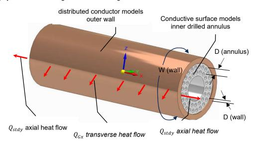
The  $Q_{stdy}$  connections can be used to transfer heat through the outer wall ends. The  $Q_{Gx}$  connection can be used to transfer heat through the outer wall cylindrical surface. One option is to attach the  $Q_{Gx}$  connector to a line heat source or line heater component with temperature or heat flux adjusted based on a separate analysis of external heat transfer.
