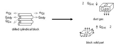
Other differences are the user-defined variables of the drilled cylindrical block, according to the above guidelines
