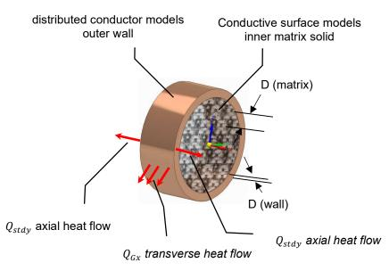
The  $Q_{stdy}$  connections can be used to transfer heat through the outer wall ends. The  $Q_{Gx}$  connection can be used to transfer heat through the outer wall cylindrical surface. One option is to attach the  $Q_{Gx}$  connector to a line heat source or line heater component with temperature or heat flux adjusted based on a separate analysis of external heat transfer.
