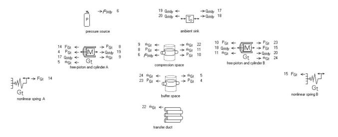
The *pressure source* establishes the *piston compression space* time-average pressure. If pasted into another model keep in mind that only one pressure source is allowed for each contiguous gas domain.
