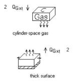
**The cylinder-space gas** is available in the Gas Domain page of the component palette available within the generic cylinder. There is also a combustion-space gas component available, which provides an internal heat source as an input variable.
