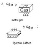
The matrix gas component is the only option in the *Gas Domain* page of the component palette inside. There is a different type of matrix gas for each parent matrix type. The rigorous surface is one of the options on the *Matrix Solids* page. Inside the matrix gas component are positive and negative gas inlets that model the mass flow rate through the end boundaries of the regenerator gas.
