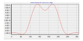
Values greater than 0 in the plots correspond to the times the values are open. The plotted variables are the interpolated views of recast inputs Frestrict, set according to math discussed in the documentation for the related model GMSingleStageSquareWaveValues.scfn.
