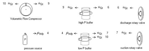
The Volumetric Flow Compressor component represents a high level abstraction that characterizes a compressor according to these inputs:
