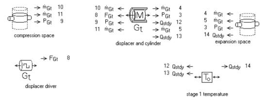
An abstract constrained-piston component (renamed displacer driver) forces the displacer to move with a defined waveform. The model contains no details about the specific mechanism that moves the displacer.
