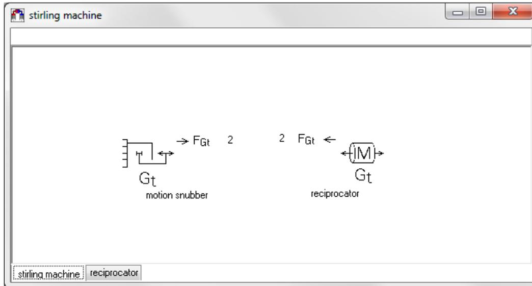
The *motion snubber* component was introduced in Sage v10 as a way to simulate the displacer of a split-cycle stirling cooler hitting end stops during the cooldown period when it is not absorbing much PV power and tends to be over-driven. This model just illustrates how the motion snubber component works without the rest of the stirling cooler components.
