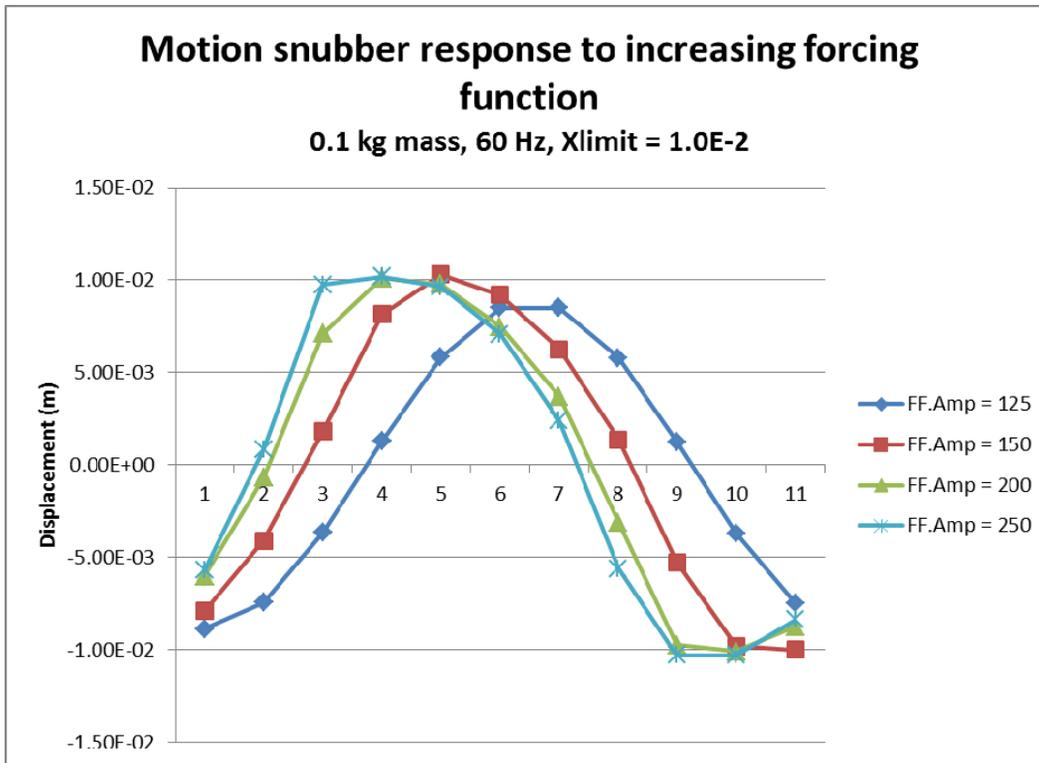
The first plot for forcing function amplitude = 125 N is essentially unrestricted free sinusoidal motion within the snubbing limits of  $\pm 0.1$  m. The next plot for FF.Amp = 125 N is just barely affected by the limits. It has a free amplitude of 0.106 m, just beyond the limits. The final two plots at FF.Amp = 200 and 250 N are increasingly overdriven. The last plot has a free amplitude of 0.176 m, as noted above but the motion snubber clamps it down within the limits.
