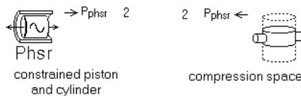
Within the *constrained piston and cylinder* component there is a constrained piston with an area attachment connected to the compression space. That area  $A$  is an independent input by default but in this case recast to  $0.25 \cdot \pi \cdot \text{Sqr}(D_{\text{shell}})$  so it automatically adjusts to the piston diameter  $D_{\text{shell}}$  input of the *constrained piston and cylinder*.
