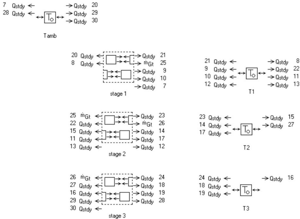
The ambient temperature ( $T_{amb}$ ) anchors the main *heat rejector*, as well as the components at the warm-end of the *stage 1* pulse tube. *Stage 1* temperature ( $T_1$ ) anchors the warm end of the *stage 2* pulse tube. The *stage 2* temperature ( $T_2$ ) could anchor the warm end of the *stage 3* pulse tube except that the connection to the bypass valve requires instead that ambient temperature ( $T_{amb}$ ) anchor it, to prevent flow between different temperatures through the valve.
