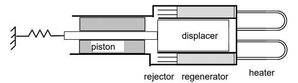
In the Sage model top level the components are arranged with cold parts on the left and hot parts on the right:
