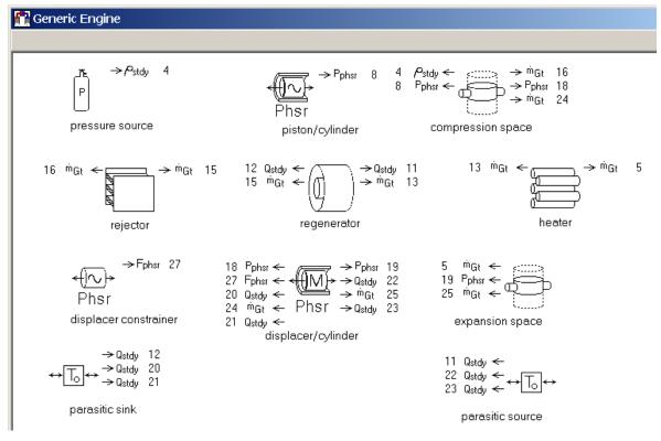
The *parasitic source* and *parasitic sink* components anchor the endpoints of the parasitic thermal conduction paths in the model. These are the regenerator pressure-wall, the
