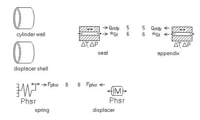
The *cylinder wall* and *displacer shell* represent the material and wall thicknesses of the fixed cylinder wall and the thin shell that insulates the displacer body from the hot expansion space. The seal models an annular clearance seal between the compression space and the *appendix*. It has an isothermal solid surface temperature inherited from input *Tinit* of the parent component. The *appendix* models the annular gas gap between
