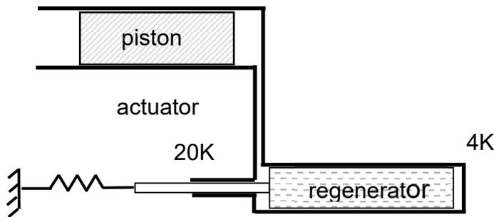
The cold-head part of the Sage model consists of a regenerative displacer capped by turbulator holes at each end that lead to a 20 K compression space and 4 K expansion space. Warmer components are at the top and colder components at the bottom in the view below:
